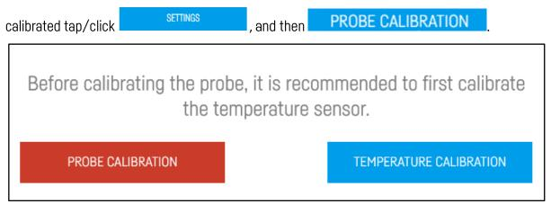
Pat dry the salinity probe and the temperature sensor, then put them both to the calibration solution 35 ppt (included in the box) or use a substitute, for example calibration solution of 53 mS/cm. The calibration fluid temperature should be exactly 25 °C (or 77 °F). In the menu select the proceed according to the steps displayed on the screen.
