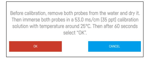
After about 60 seconds confirm the calibration process was completed by pressing the button.
